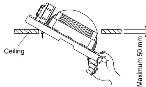
**Step 4.** Connect springs to the speaker panel to attach it.
